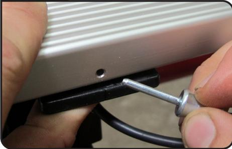
ALIGN HOLE ON FENCE WITH LINE ON PRECISION ADJUSTMENT BLOCK AND INSERT PIN TO LOCK IN PLACE
