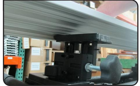
PLACE FENCE ON PRECISION ADJUSTMENT BLOCKS BY HOOKING THE BACKSIDE FIRST
