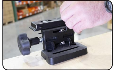
TIGHTEN ALLEN SCREWS IF THERE IS EXCESS MOVEMENT IN THE PRECISION ADJUSTMENT BLOCK
