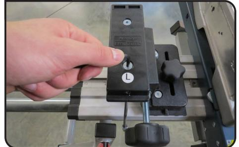
REMOVE FENCE AND UNSCREW TOP PLATE FROM BLOCK WITH INCLUDED WRENCH
