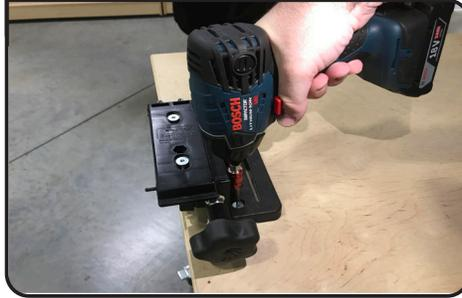
MOUNT PRECISION ADJUSTMENT BLOCKS TO WORKBENCH IN LINE WITH SAW
