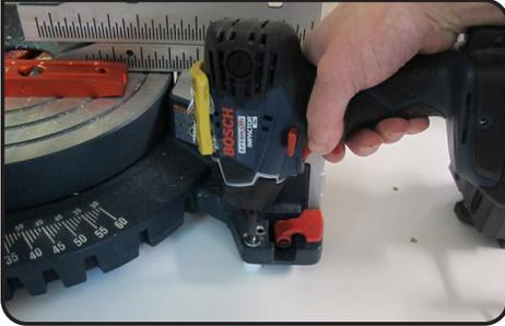
MOUNT SAW TO WORKBENCH WITH INCLUDED MOUNTING HARDWARE
